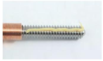
Fig. 4.1 Greasing the Leadscrew
